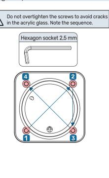
**Step 3.1:** Installing the DDC pump. Do not use the D5 ring. Note that the D5 o-ring is not suitable for the DDC. Make sure that the o-ring for the DDC pump is supplied. Place the pump directly on the adapter. Use M4 x 25 mm hexagon socket screws (not included in the scope of delivery). Tighten the screws to 2.5 Nm. Tighten the screws crosswise in the same way as for the D5 pump. (shown in the picture – step 3)
