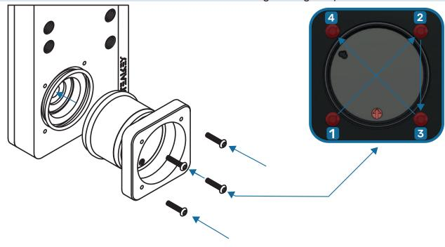
**Step 3.1:** Installing the DDC pump. Do not use the D5 ring. Note that the D5 o-ring is not suitable for the DDC. Make sure that the o-ring for the DDC pump is supplied. Place the pump directly on the adapter. Use M4 x 25 mm socket head cap screws. Tighten the screws with 2.5 Nm. Tighten the screws crosswise, in the same way as for the D5 pump. (to be seen on the picture - Step 3)
